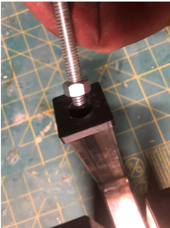
Inserting the height adjusting bolt into the foot of the center leg
