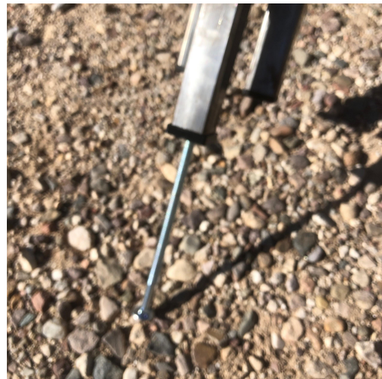
The height adjusting foot allows you to tilt the pad about 5 degrees away from spectators
