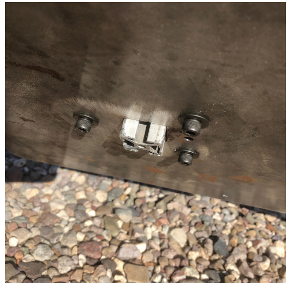
Insert the rail just far enough to secure the rail in both steel plates. Half an inch is plenty.
