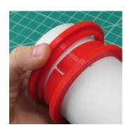
4. Squeeze the tightening ring against the self-centering ring to secure the guides in place on the tube. Using a new, sharp hobby blade, cut the tube along the edge of the guide using light pressure. Aim to cut through the tube in 2 or 3 revolutions of the tube, rather than 1 hard cut.
