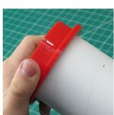
3. Leading with the narrow end, slide the tightening ring onto the narrow end of the self-centering ring, making sure to align as parallel as possible.
