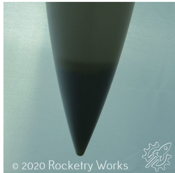
Finished photo of lead shot well secured into the tip of the nose cone
