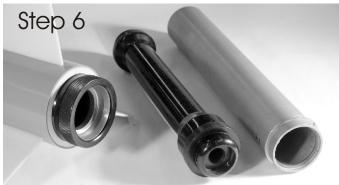
Push the motor all the way into the retainer. Apply a very small amount of grease onto the threads of the motor retainer to eliminate the potential for galling. Thread the retainer cap in place over the motor. Do not overtighten the cap. Snugging it with your thumb and two fingers is enough. That's it, go fly!
