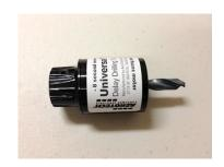
1.1 **WARNING:** Do not smoke and ensure that there are no open flames or heat sources nearby when setting the time delay. Assemble the AeroTech Universal delay drilling tool with the desired amount of delay time removal (i.e., the - 4 or - 8 seconds removal marked on the tool label) facing the exposed drill bit and motor bulkhead.
