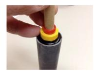
2.3 Insert the rounded end of the ejection charge cap into the ejection charge well of the bulkhead and press in completely with the end of the igniter tube or similar object.
