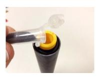
2.2 **WARNING:** Do not smoke and ensure that there are no open flames or heat sources nearby when installing the ejection charge. Open the ejection charge vial and dispense the desired amount of black powder ejection charge into the ejection charge well of the motor bulkhead. Use about ½ of the contents of the vial for 2.6" diameter rockets and smaller, and the entire vial for 3" and larger rockets. **Note:** additional ejection charge may be required for rockets exceeding 4" in diameter.
