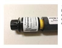
1.3 Place the open end of the tool over the motor bulkhead, hold the tool and motor firmly against each other and turn the drill knob several times clockwise until the drill knob sits flush against the drill tool body.
