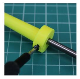
7. Insert the launch rod mount into the cross piece.
