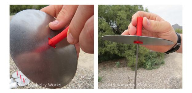
8. Pad setup is complete when all pads have the blast deflector and its mount rest around the launch rod on the launch rod mount.
