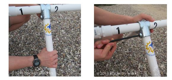
3. If you are using the pad in the taller configuration, attach the shorter leg segments to the base of the longer legs.
